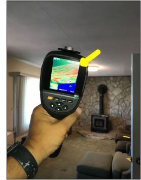
Operable heating elements.
