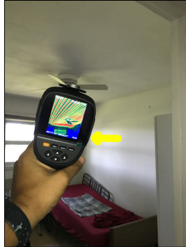
Operable heating elements.
