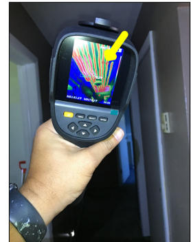
Operable heating elements.
